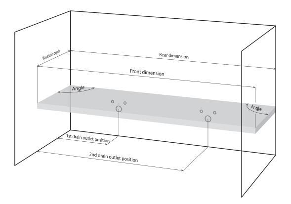
Note. All the presented dimensions must be measured in the required counter top height. Common height for washbasin counter top is 850 mm from the floor.
